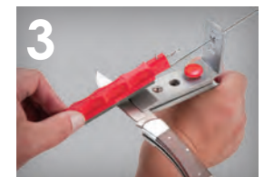
3 SHARPEN ONE SIDE, THEN FLIP
